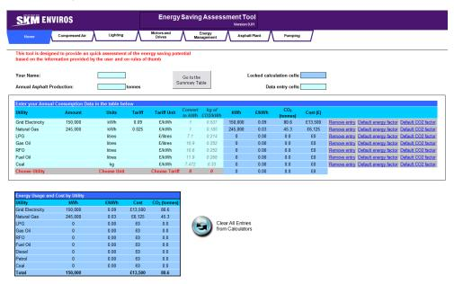
On this page the user is asked to enter the annual energy consumption figures of the site. A number of different utilities (Grid Electricity, Natural Gas, LPG, Gas Oil, RFO, Fuel Oil and Coal) are available. The user can choose in which units he wants to enter the amount of energy as well as the tariff for each utility. The available units for amount of fuel / energy and units of tariffs depend on the fuel in question. The user can remove utilities by clicking on the 'Remove entry' cell.
